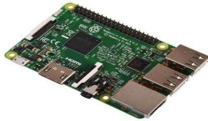
Fig 2. Raspberry Pi 3 - Model B
