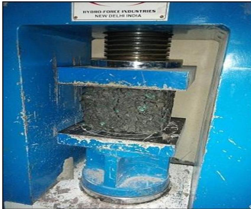
Fig 6- Compression test on DWA pervious concrete
