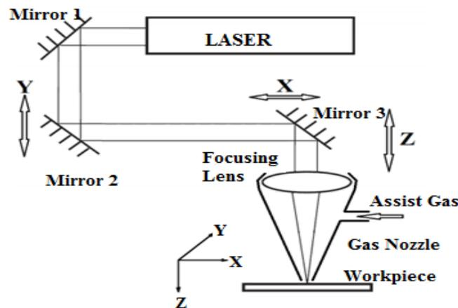
**Figure 1: Laser Drilling Process**
