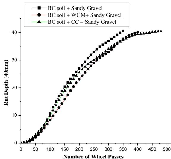
**Fig.4 Rut depth along with number of wheel passes at H/3 position coir mats.**
