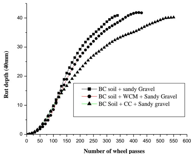
**Fig.7 Rut depth along with number of wheel passes at H/3 position coir mats.**
