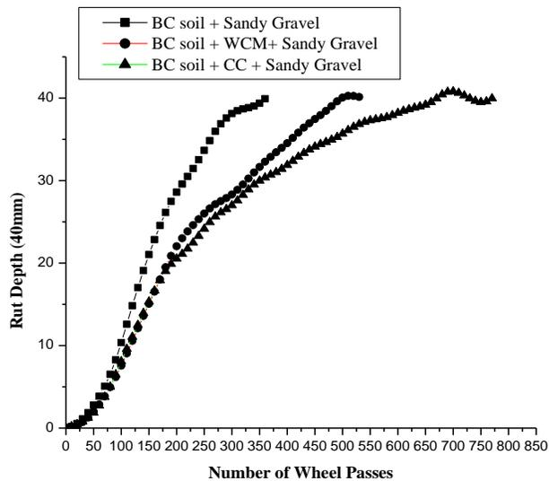
**Fig.5 Rut depth along with number of wheel passes at H/4 position coir mats.**
