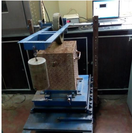
Fig.2 Wheel tracking test apparatus with 400mm mould setup
