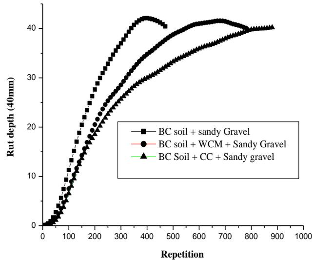
**Fig.6 Rut depth along with number of wheel passes at H/2 position coir mats.**
