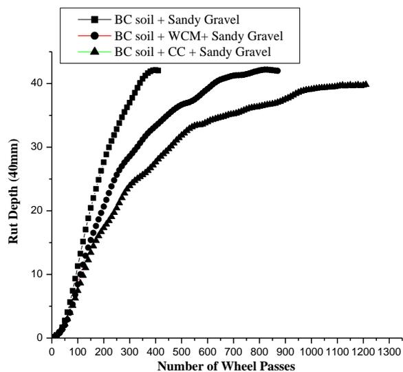
**Fig.3 Rut depth along with number of wheel passes at H/2 position coir mats.**
