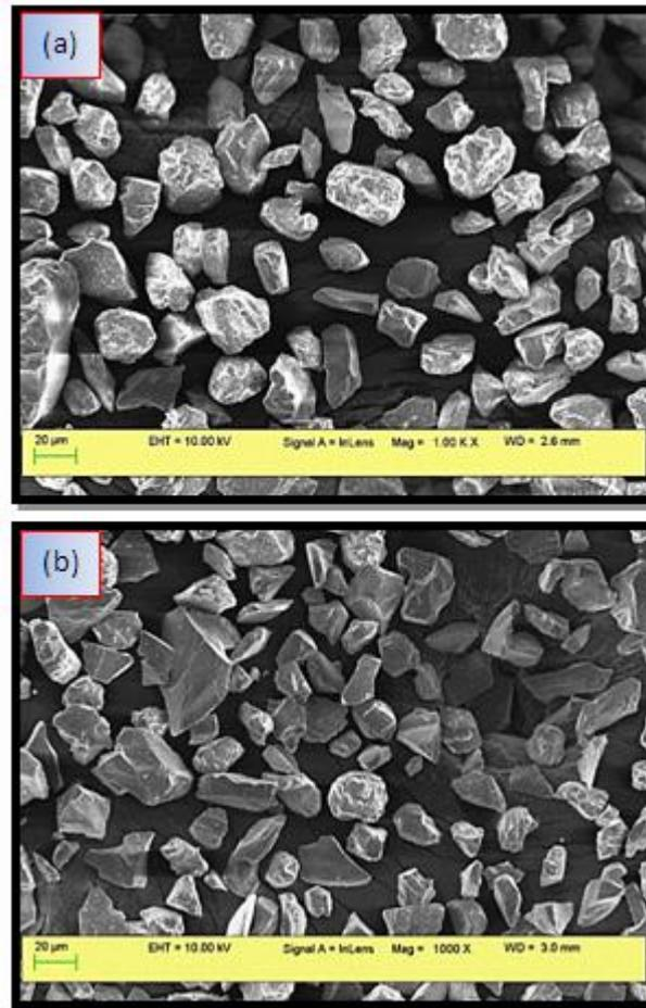
**Fig. 4: powder sem images of Al<sub>2</sub>O<sub>3</sub>: TiO<sub>2</sub> with composition (a) 87:13 and (b) 50:50**
