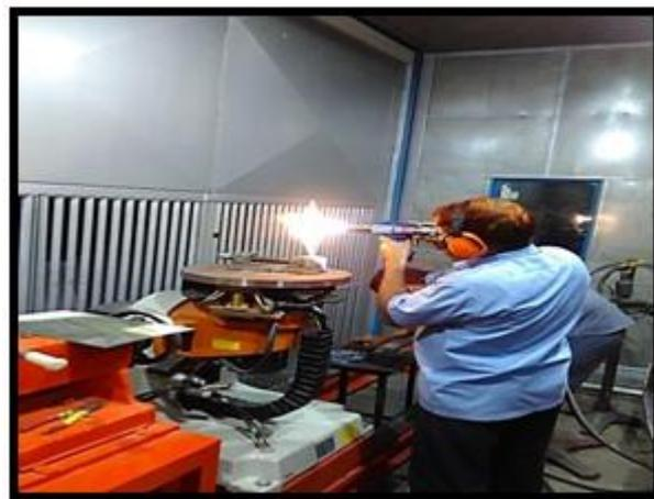
**Fig. 2 : experimental flame spray at MEC Jodhpur**
