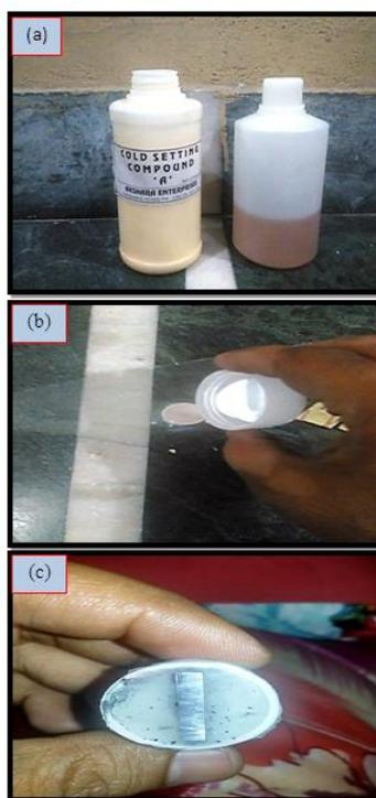
**Fig.6: sample mounting process for cross sectional sem**
