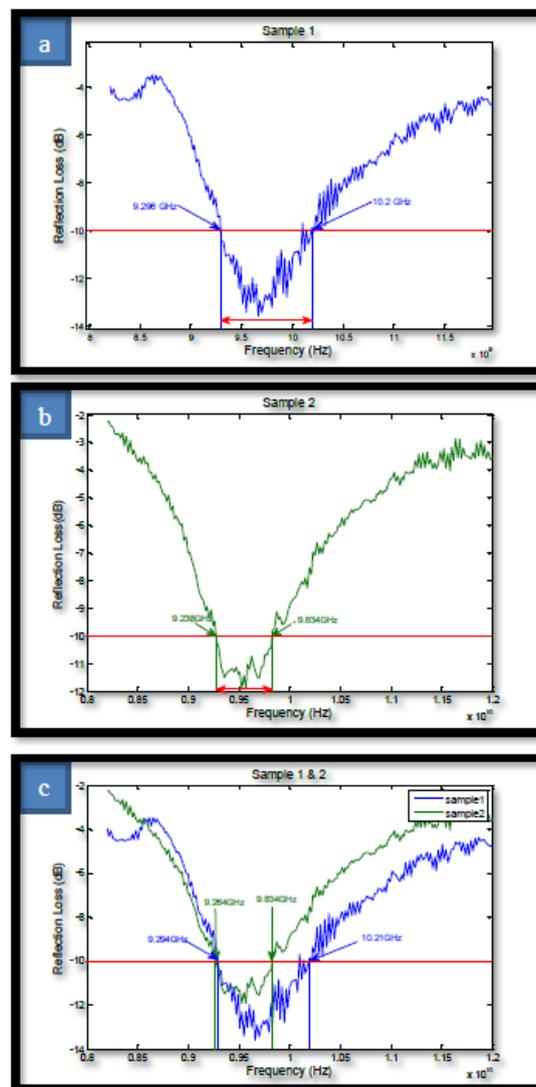
**Fig. 9: the reflection-loss spectra S<sub>11</sub>: (a) sample 1 (b) sample 2 (c) combined sample 1 & 2**
