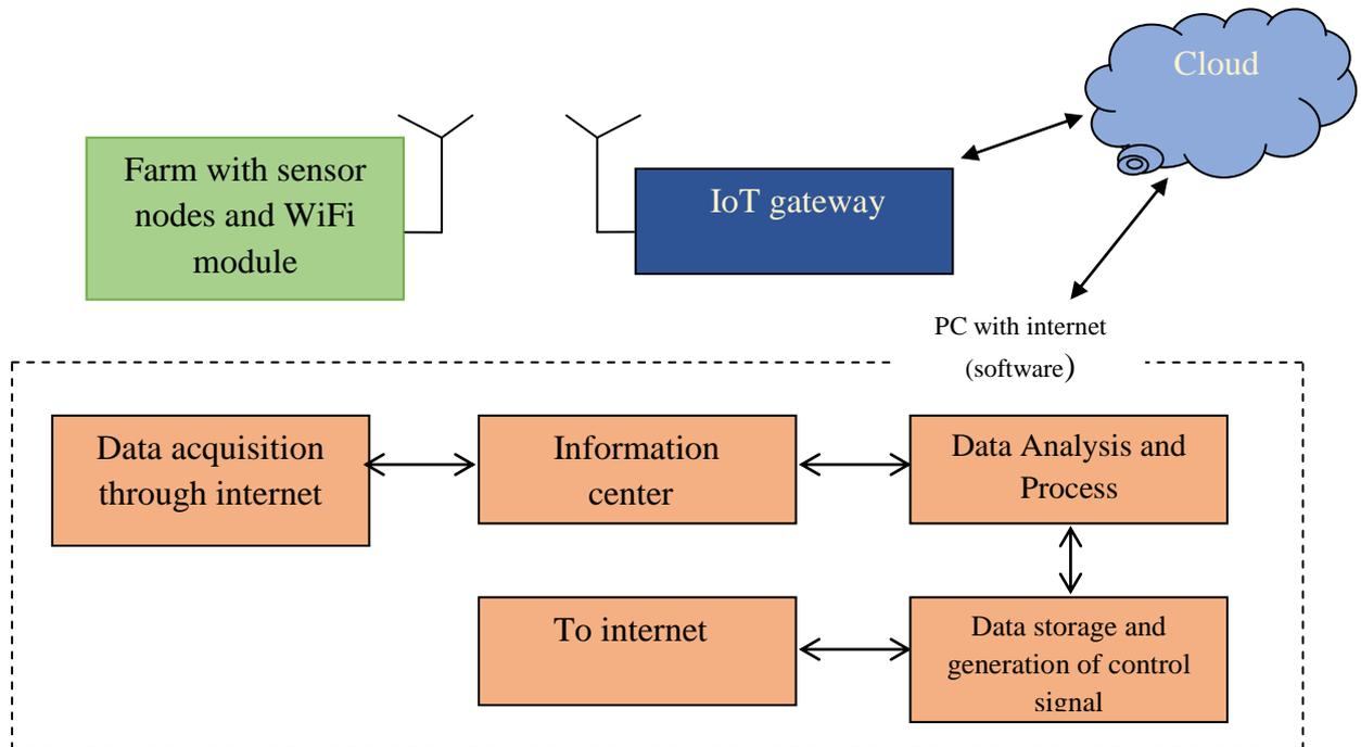
**Fig 1: Generalized block diagram of proposed system**
