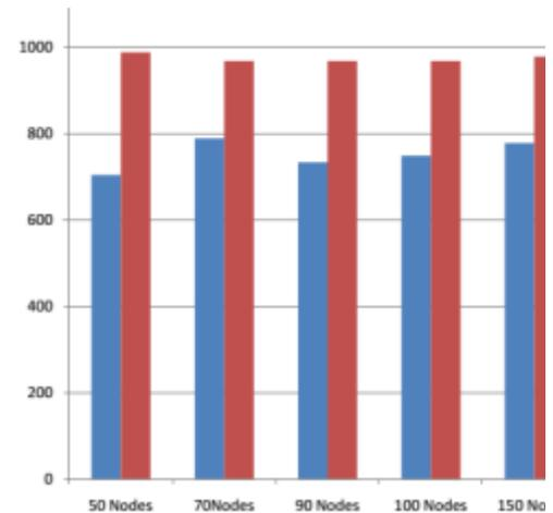
3.2: Number of Application packets received. Transmission power is 50.69mW, and 5 source nodes in the network
