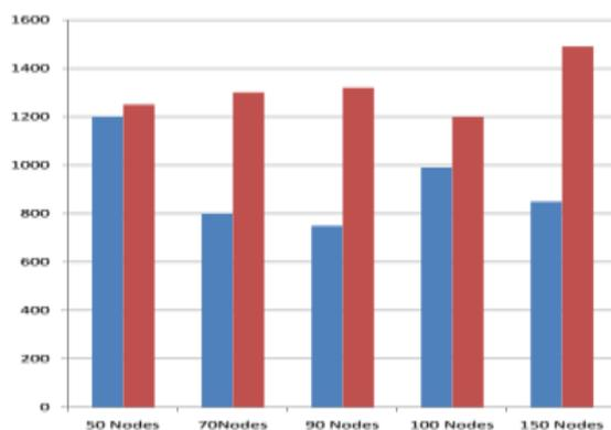
3.5: Number of Application packets received. Transmission power is 42.24mW, and 10 source nodes in the network
