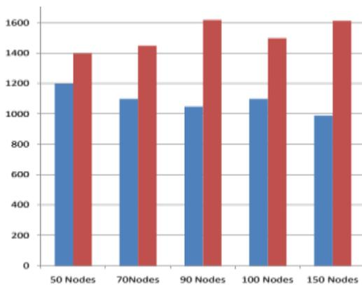
3.3: Number of Application packets received. Transmission power is 50.69mW, and 10 source nodes in the network
