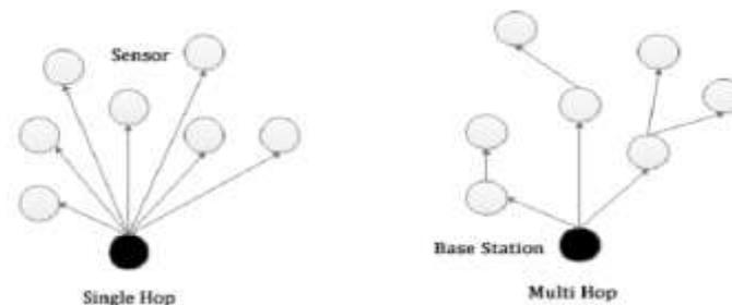
**Figure 1: Single Hop and Multi Hop Communication.[5]**
