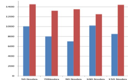
3.4: Number of Application packets received. Transmission power is 42.24mW, and 5 source nodes in the network
