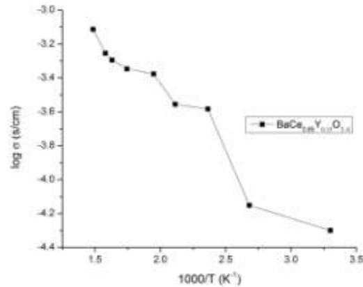
Fig. 7. Arrhenius plot of conductivity in air for samples sintered at 1300°C/5h BaCe<sub>0.85</sub>Y<sub>0.15</sub>O<sub>3</sub> oxides.
