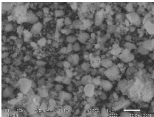
Fig.3. SEM morphologies of sintered ( $1300^{\circ}\text{C}/5\text{h}$ )  $\text{BaCe}_{0.85}\text{Y}_{0.15}\text{O}_3$  oxides.
