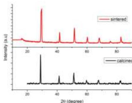
Fig. 2 XRD patterns of calcined ( $1000^{\circ}\text{C}$ ) and sintered  $\text{BaCe}_{0.85}\text{Y}_{0.15}\text{O}_3$  ( $1300^{\circ}\text{C}$ ) oxides.
