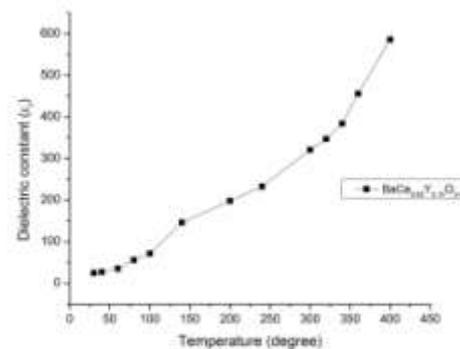
Fig. 9. Variation of Dielectric constant with Temperature of sintered (1300°C/5h) BaCe<sub>0.85</sub>Y<sub>0.15</sub>O<sub>3</sub> oxide.
