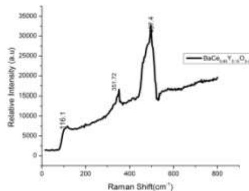
**Fig. 5. Raman spectra of sintered (1300°C/5h)  $\text{BaCe}_{0.85}\text{Y}_{0.15}\text{O}_3$  oxides.**
