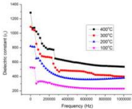
Fig 8. Dielectric constant vs frequency plot of sintered (1300°C/5h) BaCe<sub>0.85</sub>Y<sub>0.15</sub>O<sub>3</sub> oxides.
