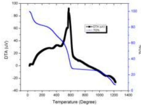
**Fig. 1 TG-DTA curves of BaCe<sub>0.85</sub>Y<sub>0.15</sub>O<sub>3</sub> powder preheated at 250°C for 24h.**
