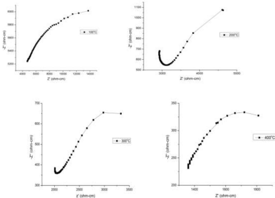
**Fig 6 Nyquist plots at various temperature in air for sintered (1300°C) BaCe<sub>0.85</sub>Y<sub>0.15</sub>O<sub>3</sub> oxides.**
