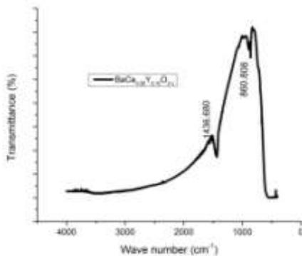
**Fig. 4. FTIR spectra of sintered (1300°C/5h)  $\text{BaCe}_{0.85}\text{Y}_{0.15}\text{O}_3$  oxides.**
