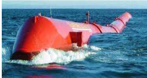
Figure 2: Pelamis wave energy converter [Adopted from www.buildipedia.com ]
