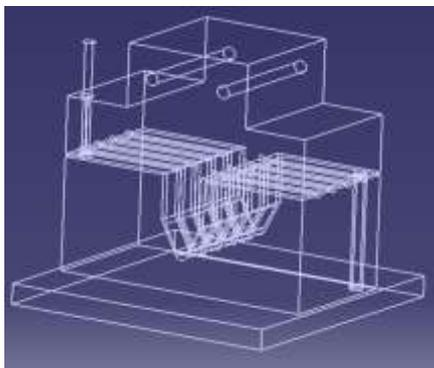
**Fig 5.4.3 3-D Model of designed Die and Punch**
