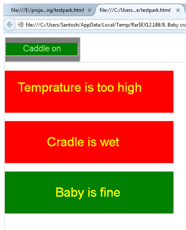
Fig.4 System output shows high temperature and wetness detection
