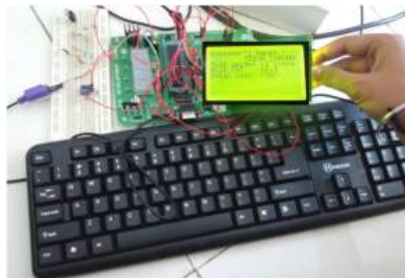
Fig. 4 Interfacing keyboard and GLCD with PIC
