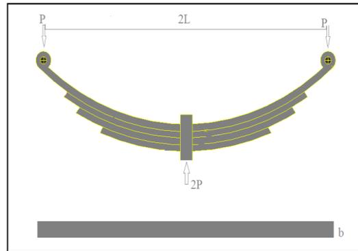
**Fig 2.1 Beam Theory for Leaf Spring**
