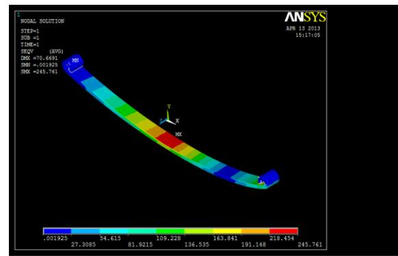
Fig 2.3: Stresses induced in composite leaf spring
