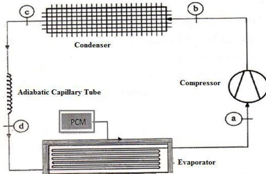
**Fig.1 Line Diagram of Refrigeration Cycle**
