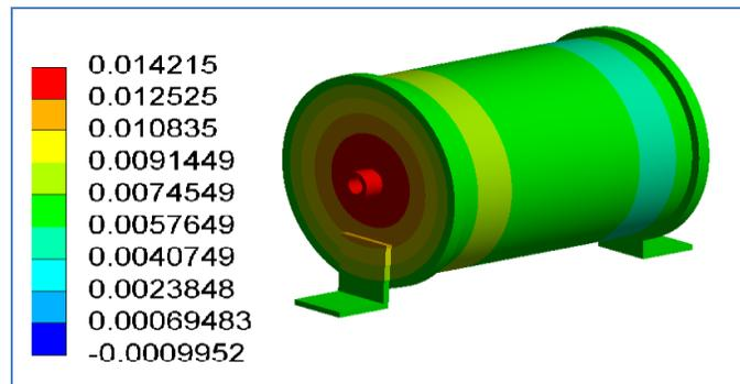
Figure (3) deformation (Strain in E2) in 0.00142 mm.
