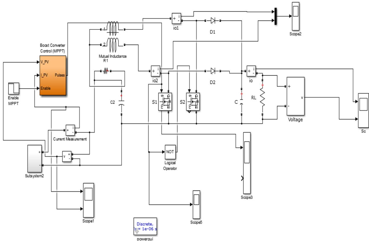
**Fig.3 MATLAB modeling of IBC with PV input**
