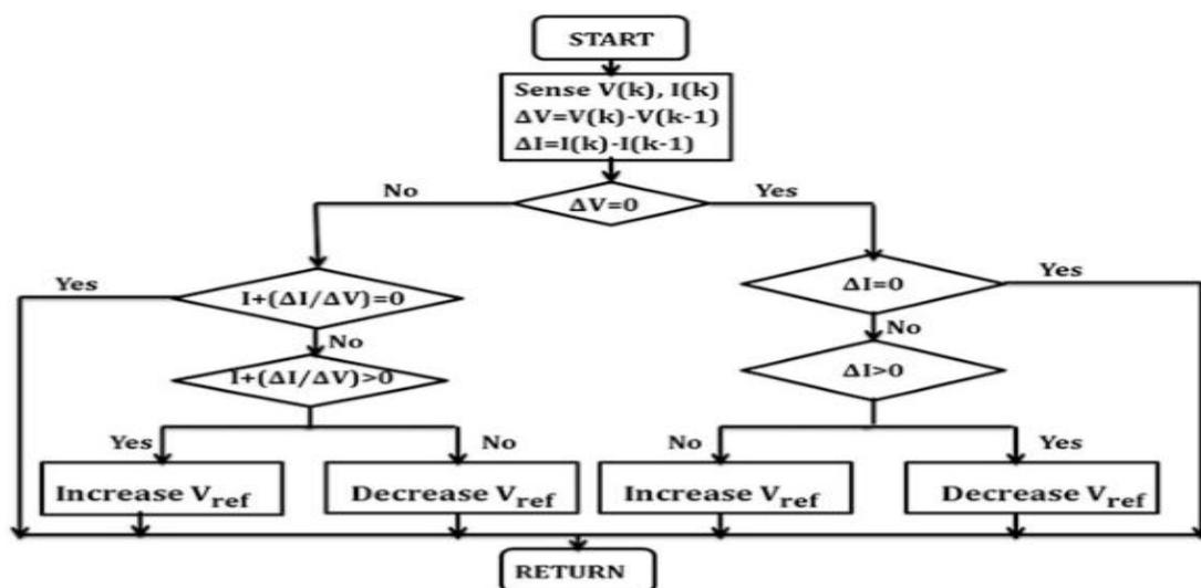
**Fig.2 Flow-chart of Incremental Conductance (InCond) algorithm**
