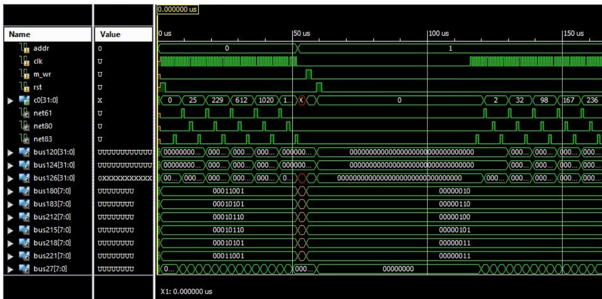
Fig. 7(b) Simulation Result of Polyphase Decimator In Transposed Form With FSU
