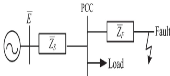
**Fig (2): Single-phase model for voltage sag at the PCC**
