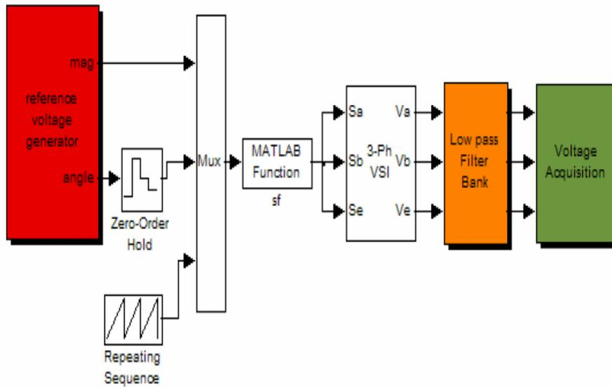
Fig (3): Reference Voltage Generation in the Form of Vector
