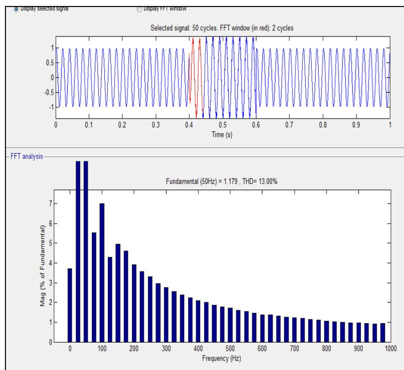
**Fig.(10): FFT analysis during 3-Ø fault With RVG**
