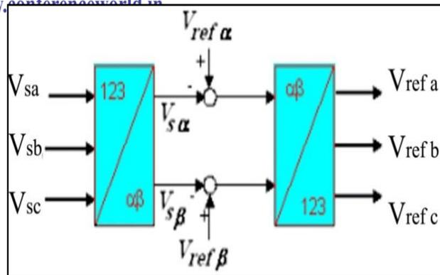
**Fig (5) Principle of the Voltage Reference Frame**
