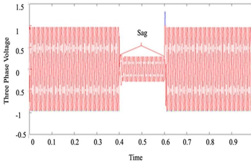
Fig.(7): 3- $\phi$  Voltage at Load Point, With 3- $\phi$  Fault, Without DVR
