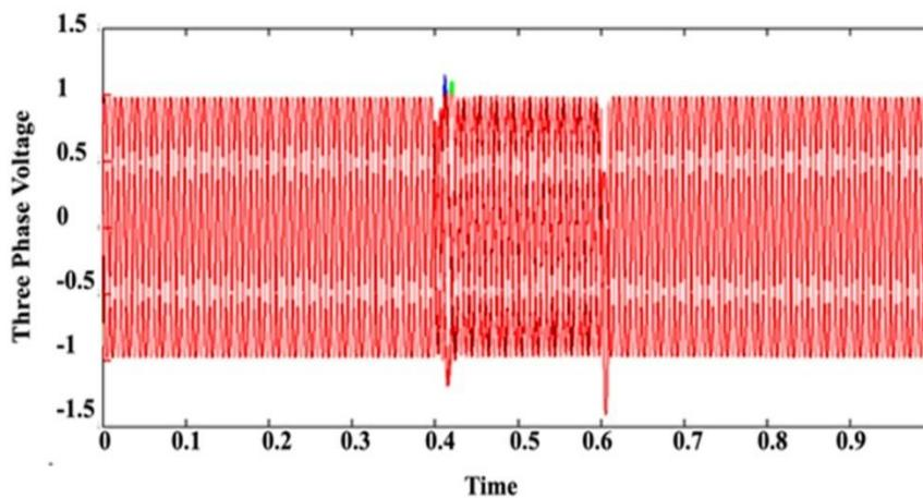
Fig.(8): 3- $\phi$  Voltage at Load Point, With 3- $\phi$  Fault, With DVR RVG
