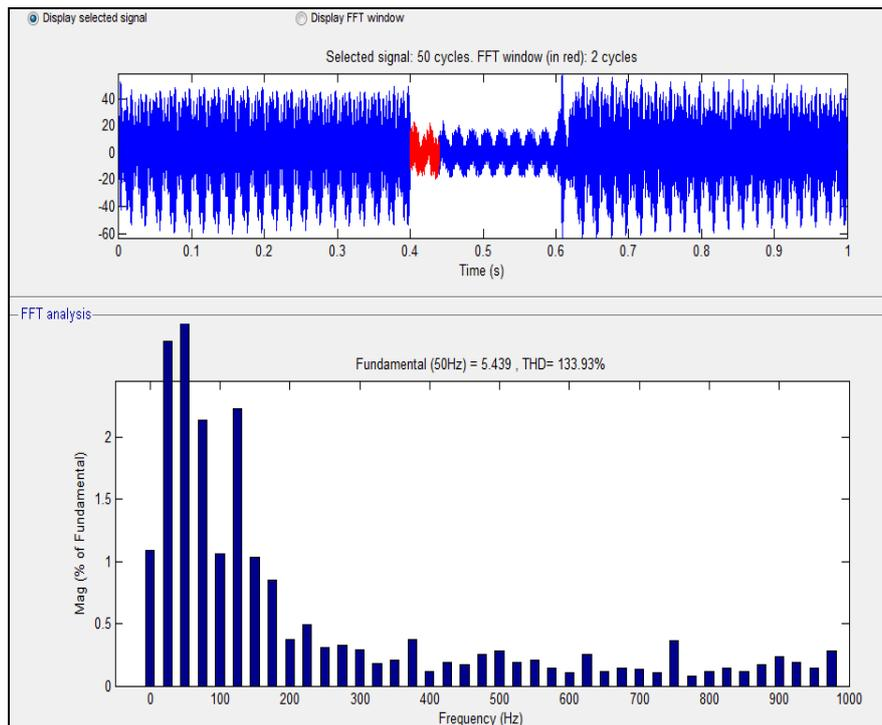
**Fig.(9): FFT analysis during 3-Ø fault Without RVG**
