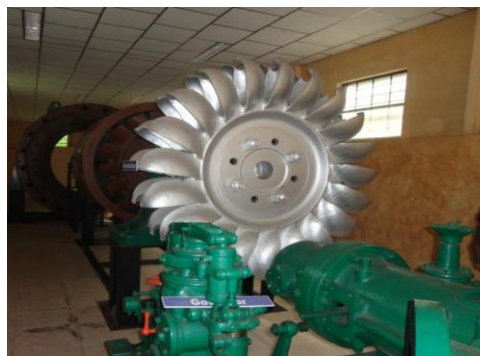
Fig 1. Pelton Runner Model
