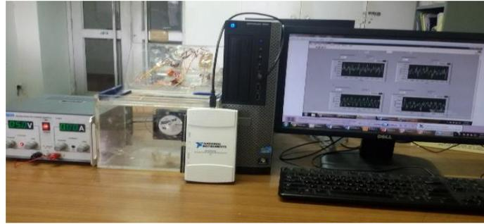
Fig. 4 Real Time Monitoring Set-up
