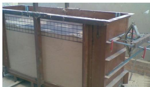
**Fig. 3 Sand container and lateral stressing mechanism**
