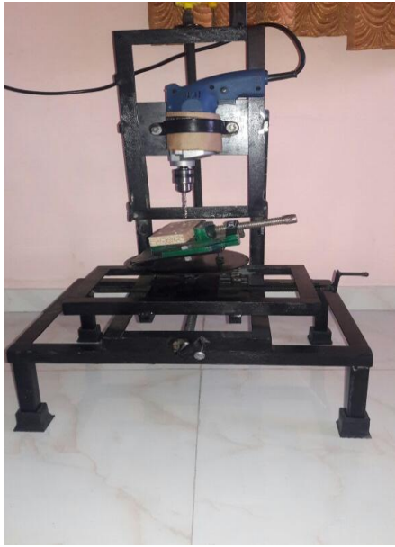
Fig: working model of 6-way drilling machine
