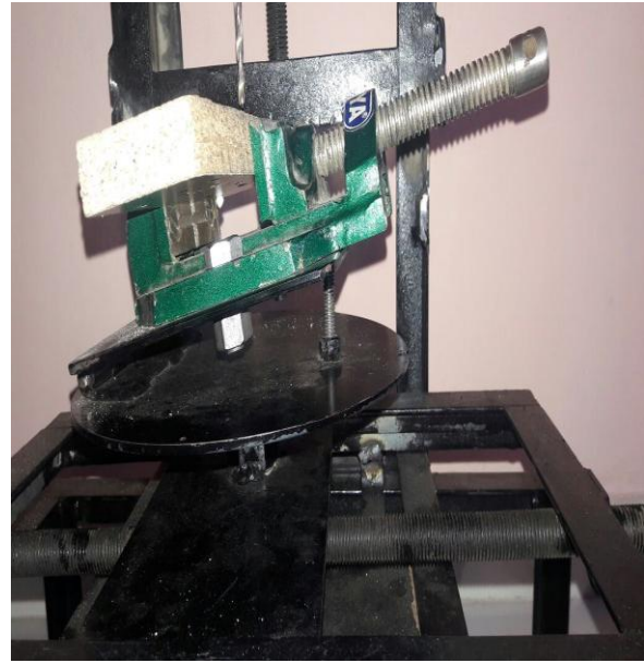
Fig: inclination of fixture
