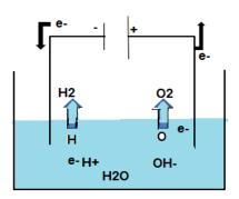
Electrolysis process takes place in fuel cell
