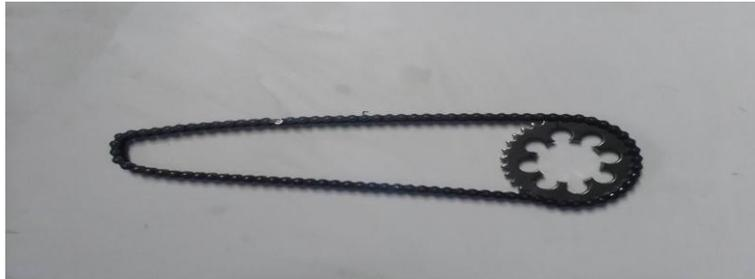
Chain drive is provided to avoid the slippage as the motor has to feed the rod which is heavy at low rpm. So chain drive was the best suited option among various types of drives.
