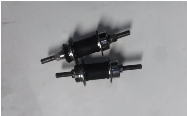
Rollers are provided for the frictionless movement of the rod so that the bar can be easily fed or pushed with less power.
