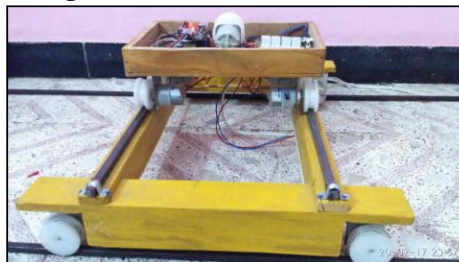
Figure 5.3.2 Hoist model side view
