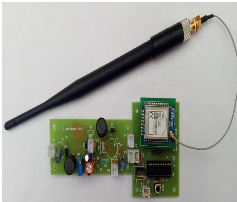
Fig 7.2 Hardware of converters, microcontroller and ZigBee
