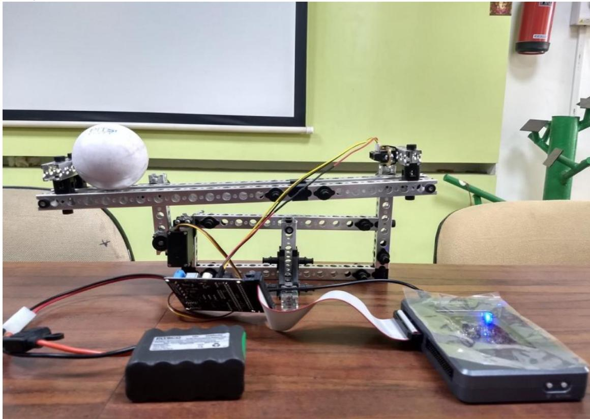
**Figure 5:** complete setup of the single-joint robotic arm
