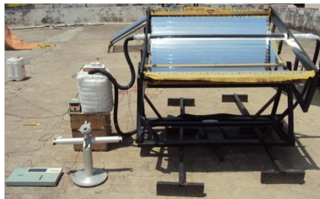
Figure 1: Experimental set up (Parabolic trough collector)
