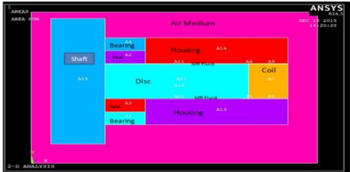
Fig 4. Two dimensional axi-symmetric model of MR brake.
