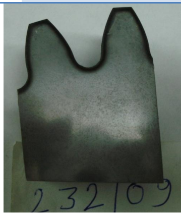
Fig.3 Photograph showing case depth of sample no.232/09/2.
