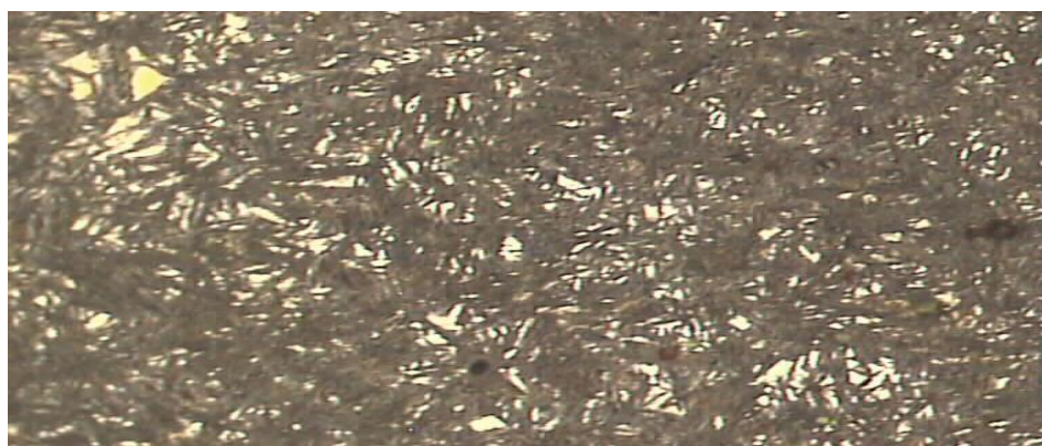
Fig.4 Photomicrograph showing tempered martensite structure in X500 sample no.232/09/1 (cam gear).
