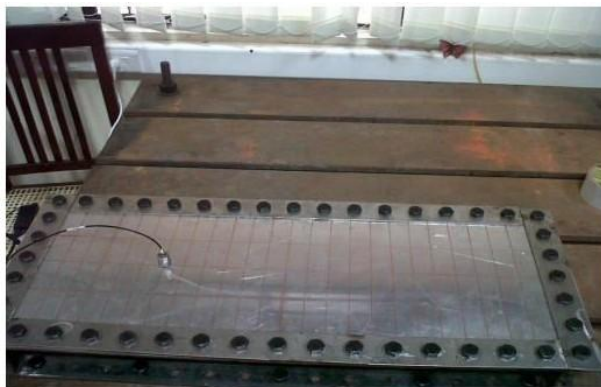
Fig1: Accelerometer mounted on the aluminum plate with clamped B.C
