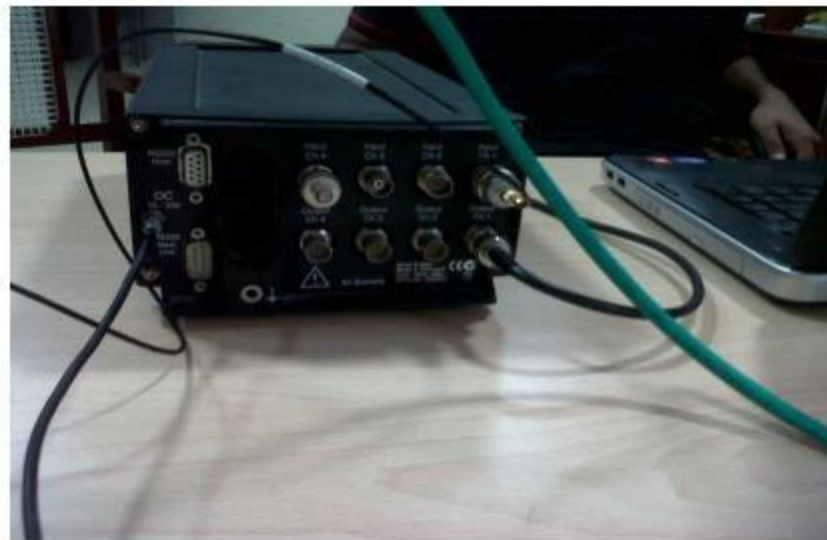
Fig2: Connection of response of accelerometer into the input channel1 and the connection of BNC Cable, going into the LAN-XI, from the output channel 1
