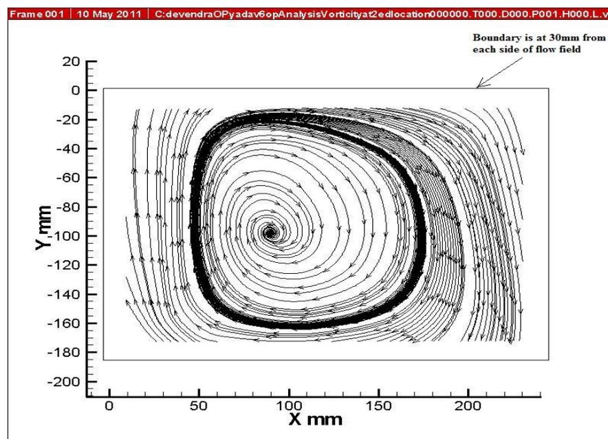
Figure:9 stream line for average velocity field at section-2
