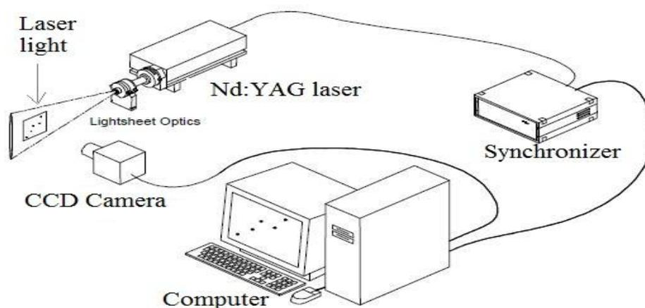
Figure:2 Particle image velocimetry (PIV) system
