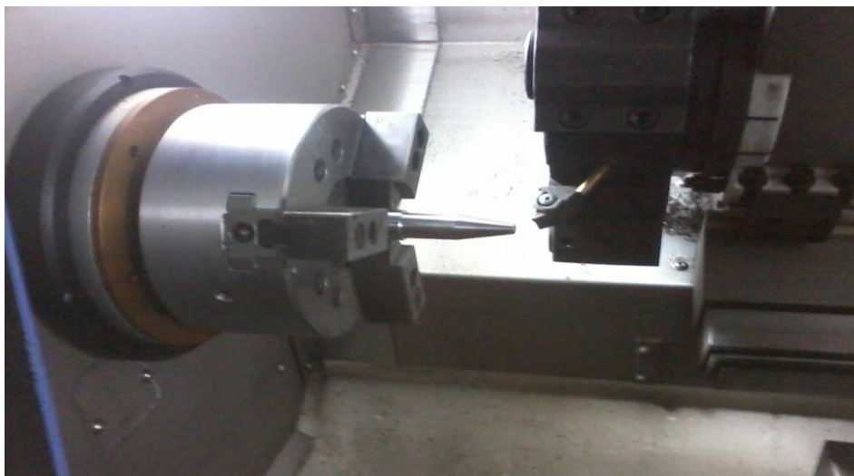
Fig .4 Machining of Zinc Metal Specimen used
