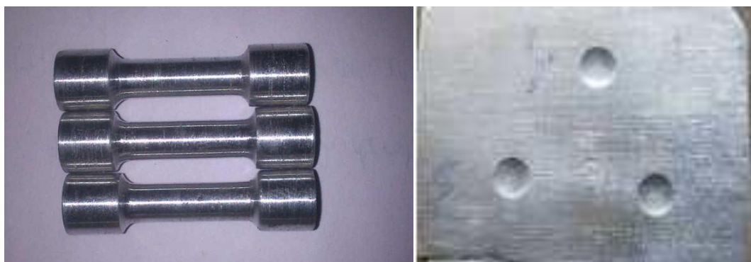
Figure 1 (a) Tensile Specimens, (b) Indentation on specimen after hardness test
