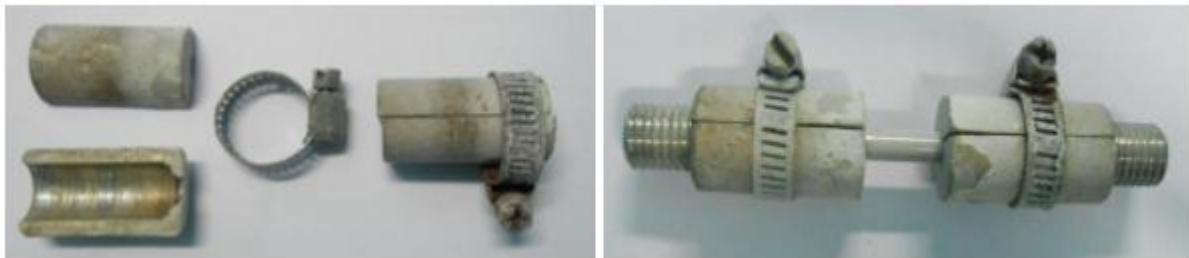
Fig.1: Adaptors used for covering the radial and threaded portion of the LCF sample
