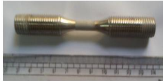
Fig 3: NaCl salt coated LCF sample
