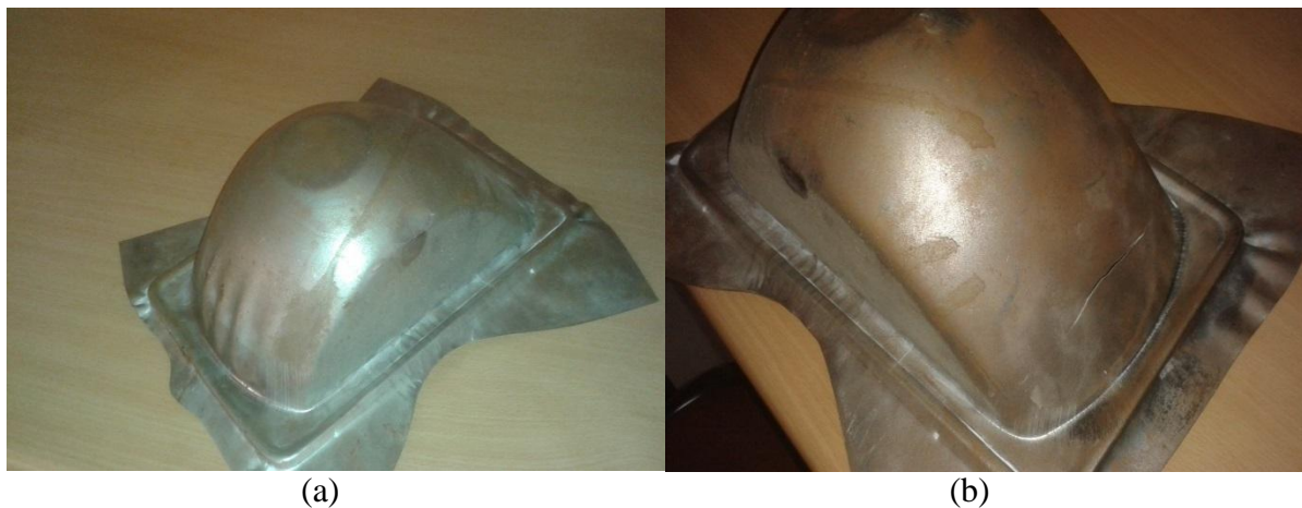
FIGURE 2.1 Defected Part having (a) Wrinkling and (b) Tearing
