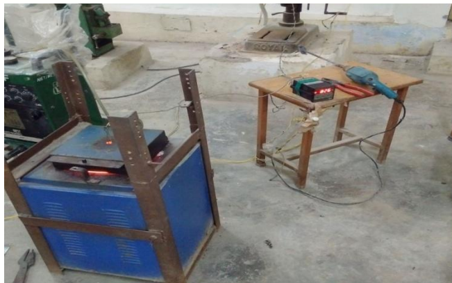
Fig. 1 Stir Casting equipment
