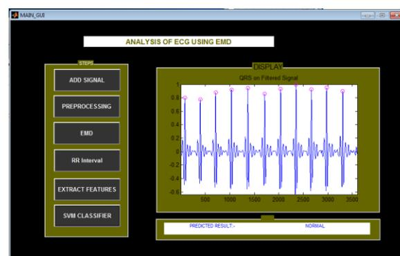
The SVM classifier (neural network) used for matching observed data to trained data and monitor that the signal is normal or abnormal. The accurate ECG data send to the IOT cloud then the measured data provide to the hospitals or relatives or emergencies numbers in emergencies.
