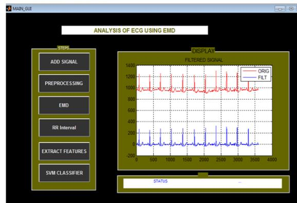
The RR-interval signals are nonlinear and non-stationary in nature. Hence linear methods may not be able to capture the hidden information present in the signal. In this paper, a new nonlinear method based on empirical mode De-composition (EMD) is proposed to discriminate between abnormal and normal RR-interval signal.
