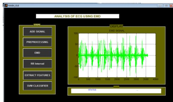
The mean frequency parameter using Fourier Bessel series expansion (MFFB) and the two bandwidth parameters namely, amplitude modulation bandwidth (BAM) and frequency modulation bandwidth (BFM) extracted from the intrinsic mode functions (IMFs) obtained from the EMD of RR-interval signals are used to discriminate the two groups.
