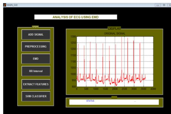
EMD used after pre-processing for accuracy. for R-R interval Pam & Tompkins algorithm applied here.
