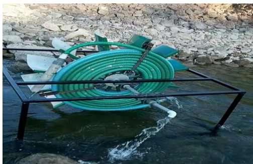
Fig. spiral tube water wheel pump
