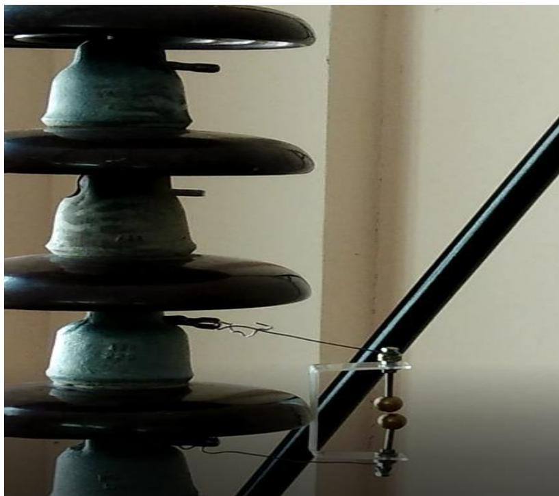
Fig.2 Arrangement of voltage distribution without guard rings
