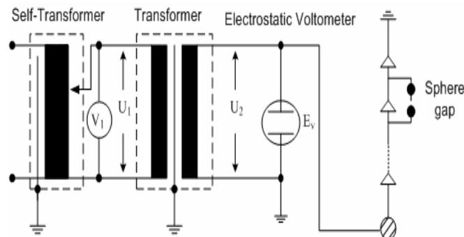
Fig.1: Measurement of Voltage Distribution by sphere gap
