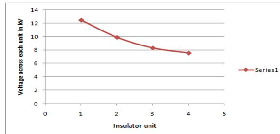
Fig. 6: Graph between voltage across each unit and given insulator value
