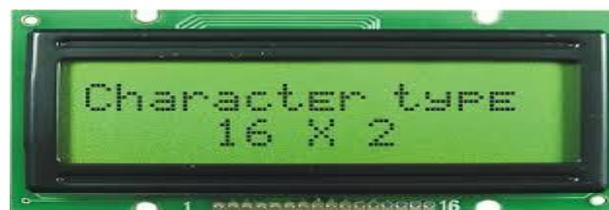
Fig 7: 16x2 LCD display
