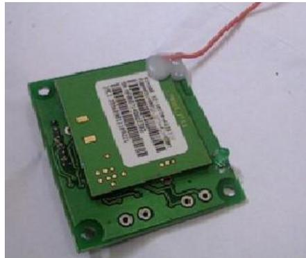
Figure 4: GSM Modem
