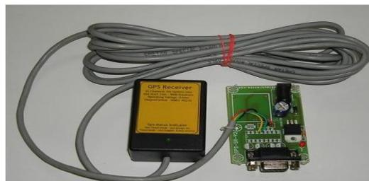
Figure 5: GPS Modem
