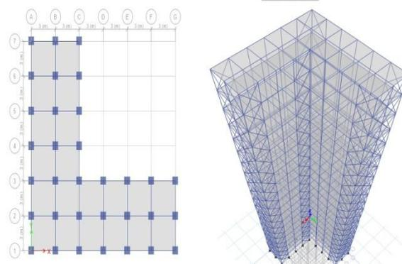
Fig. 1. a)Plan of Moment Resisting Frame L-Section building
