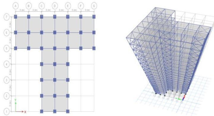
Fig. 1. a)Plan of Moment Resisting Frame C-Section building
