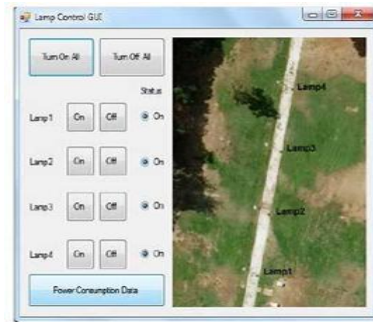
Figure-6: Exemplary GUI of the lighting system.
