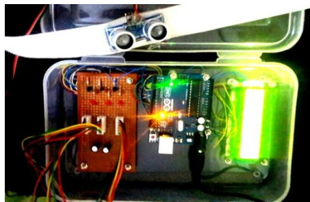
Fig 4: PCB showing Arduino Uno and interfaced components.
