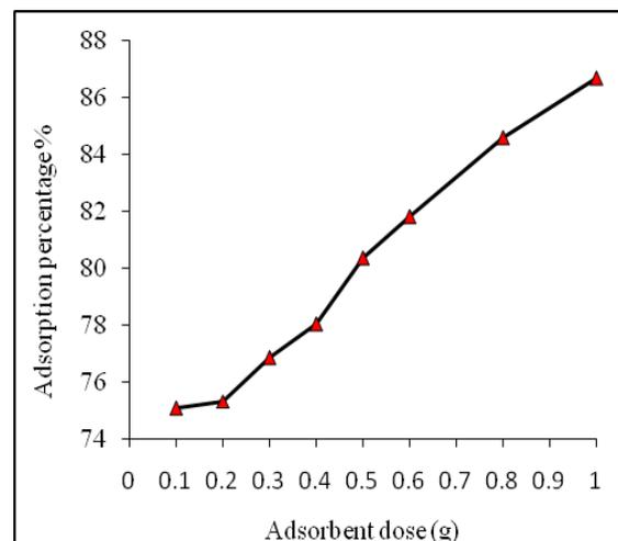
Fig. 4 Effect of dose on adsorption of Pb(II)
