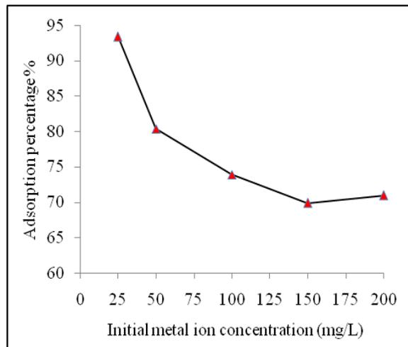
Fig. 2 Effect of concentration on adsorption of Pb(II)
