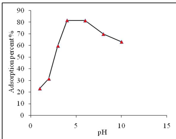
Fig. 1 Effect of pH on adsorption of Pb(II)
