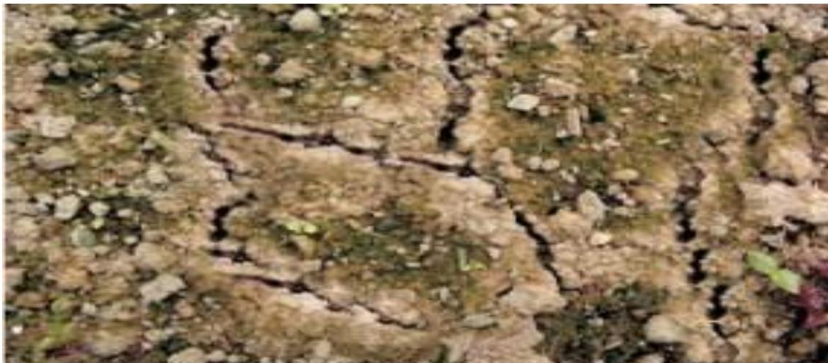
Figure 2: Typical Cracks in Black Cotton Soil in a Dried State
