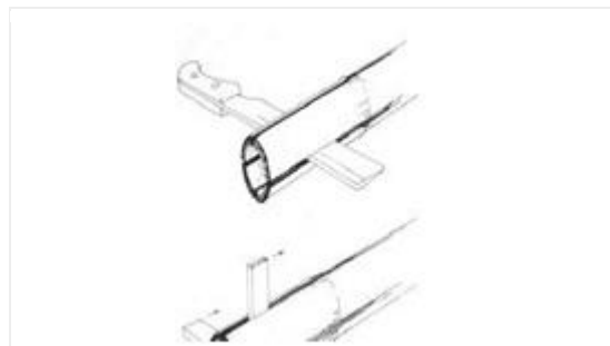
Fig 2(a) Splitting of a bamboo cane.
