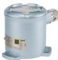
The SES70 Intelligent Earthquake Sensor detects the acceleration caused by an earthquake using a small built-in accelerometer and then calculates and outputs the synthetic acceleration, the estimated Japan Meteorological Agency seismic intensity scale (shindo scale) value, and the SI value, which is an estimation of damage to structures caused by earthquake motion.
