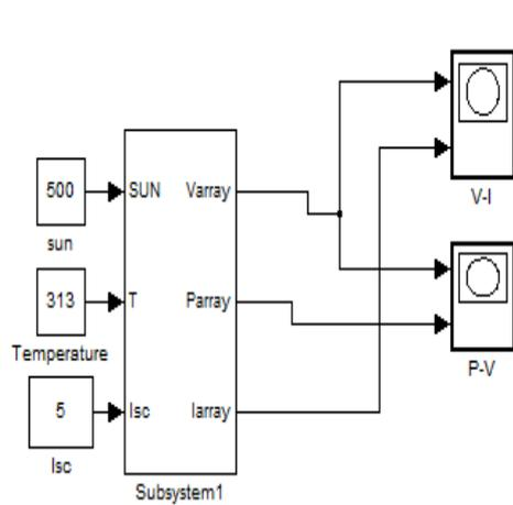
Figure 2. The Simulink model of the solar cell
